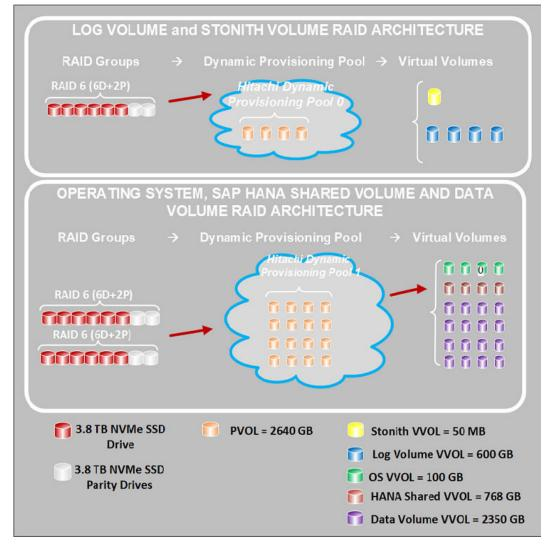
Build the Hitachi Virtual Storage Platform E1090 with the components as shown in the following table for 4 nodes, 8 nodes, 12 nodes, or 16 nodes.
