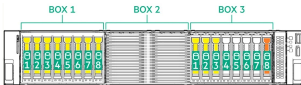
Hitachi Advanced Server HA840 G3 with used Internal Disks and Hot spare drive (Front)
