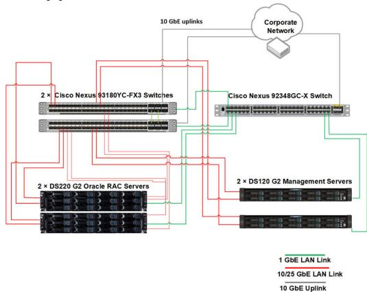
The following figure shows the IP network switch connection.
